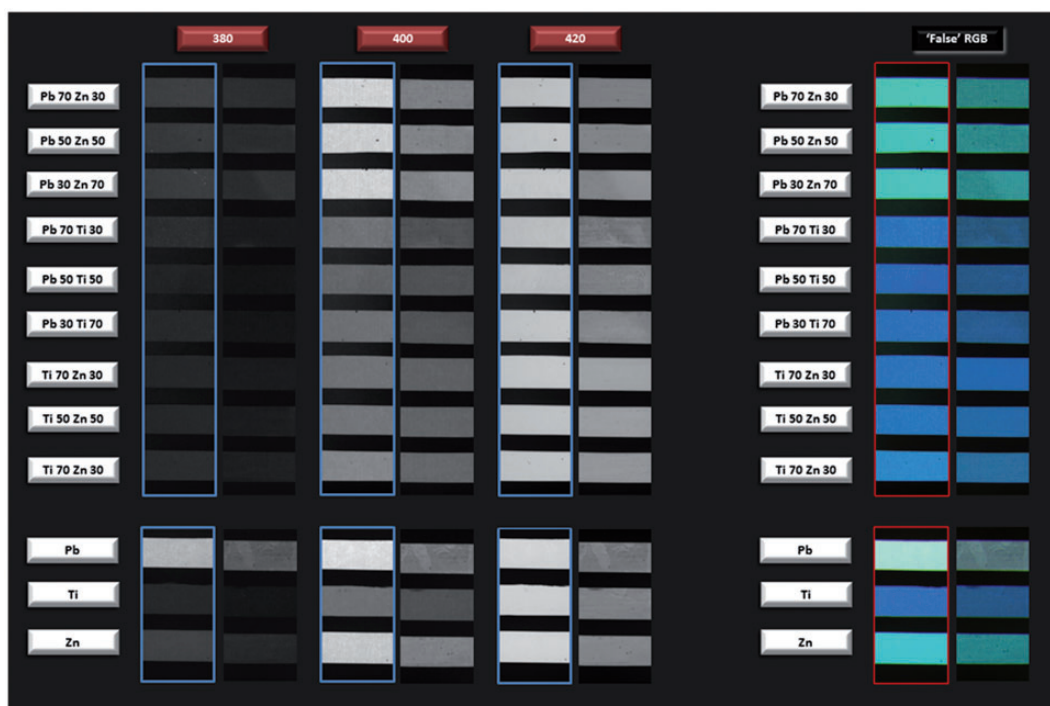
Figure 7. Multispectral images at 380 nm (R), 400 nm (G), and 420 nm (B) of the white mixtures (left panel) and “false” RGB combination of the same images. The yolk samples are framed in blue in the multispectral images and in red in the false RGB image.
