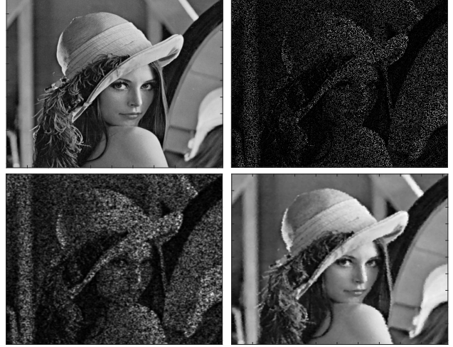
Figure 2. Top left: The famous Lena-image, top right the image has been degraded to a grey-level test image only containing 20% of the original information. Bottom left: Interpolation using standard convolution with a normalized smoothing filter (see Figure 1). Bottom right: Interpolation using normalized convolution with the same filter as applicability function.
