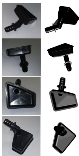
Figure 13: Estimating the object pose from real images. Left: the real image. Right: the rendered estimated pose. The estimation average accuracy reaches 22°.
