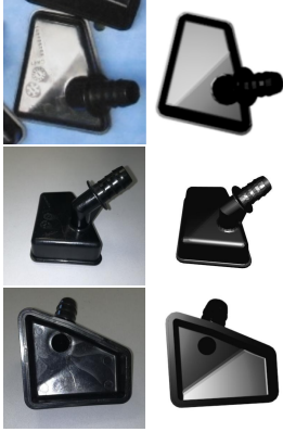
Figure 5: Relevant scene parameters can render realistic views of the part. Left: the real image pose. Right: the rendered approximated pose.
