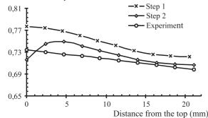
Fig. 3. Axial relative density profile over the height of the tablet. Compaction of 2.75 g of MCC up to 60 Mpa.
