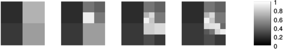
FIGURE 2. Principle of the multiresolution algorithm: compute an image with coarse pixels, then refine sets of intense pixels, iteratively.
