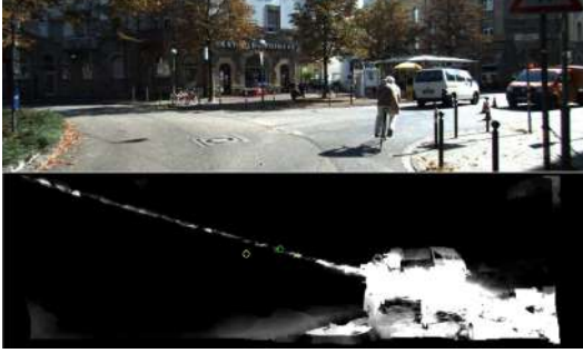
Figure 3: Example of unstable detection result caused by unmodified projective depth calculation. Top: Original image. Bottom: Moving pixels detected by Eq.7
