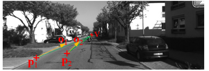
Fig. 7. Example of a road image with two marked voters p_1 and p_2 with estimated orientation of o_1 and o_2 , respectively.
