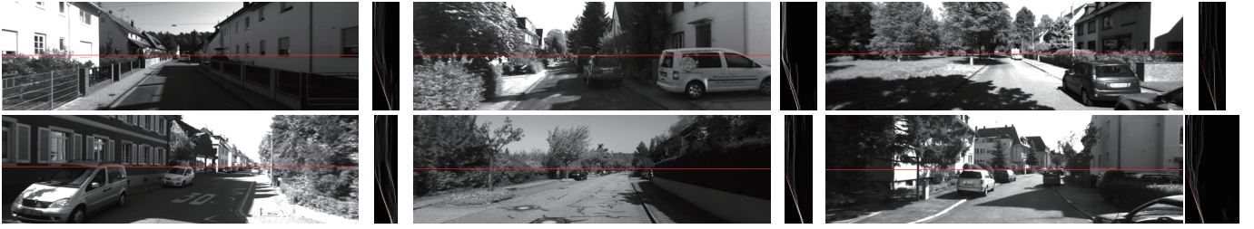
Fig. 5. Detected horizons across different scenes based on v-disparity map.
