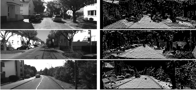
Fig. 8. Example of the gray-scale images (left) and the corresponding disparity feature cost map (right). The disparity feature cost in the curb region is obviously lower than that of its surrounding road region.
