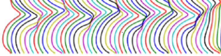
Figure 6: Successive front positions provided by the Sivashinsky DL-model equation triggered by "combustion holes"
