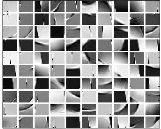
Fig. 2. Atoms of the dictionary learnt from the displacements of the LADdist sequence (Section V-D), patch size w = 16 \times 16 , maximum number of non-zero coefficients K = 5 .
