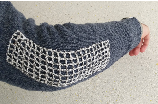
Fig. 2: The piezo-resistive sensor integrated in the sweater.
