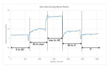
Fig. 4: Example of noise on raw data from textile sensor.
