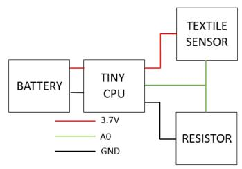
Fig. 3: Hardware architecture of the electronic system based on TinyDuino platform.
