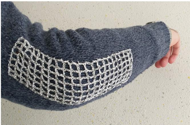
Fig. 2: The piezo-resistive sensor integrated in the sweater.
