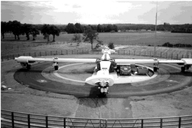
Figure 1. View of the LCPC fatigue test track.
