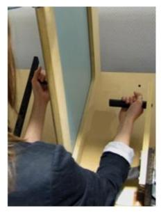
Figure 1. Illustration of the experimental setup for the kinesthetic mirror illusion task. The participant sat at a table and faced a box compartmentalized by a vertical mirror. Left: the participant's left arm was supported by a motorized manipulandum that could flex the arm. Visible to the participant, the vertical mirror reflected the image of their left arm. Right: invisible to the participant, their right arm was supported by a static manipulandum and held at a 15° angle.
