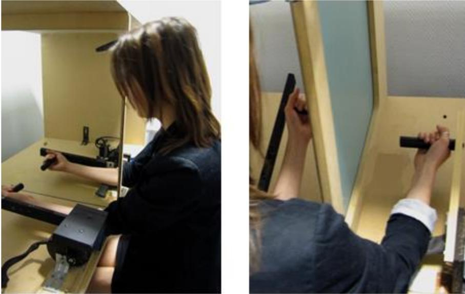
*Figure 1. Illustration of the experimental setup for the kinesthetic mirror illusion task. The participant sat at a table and faced a box compartmentalized by a vertical mirror. Left: the participant's left arm was supported by a motorized manipulandum that could flex the arm. Visible to the participant, the vertical mirror reflected the image of their left arm. Right: invisible to the participant, their right arm was supported by a static manipulandum and held at a 15° angle.*
