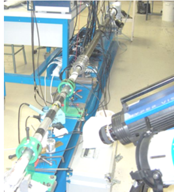
Fig. 7 (a) Principle of the spalling test. (b) View of the experimental setup [62]
