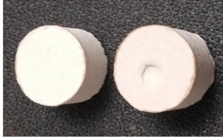
Figure 2: Sample used in the *in-situ* laboratory experiment. Plasterboard sample (left) before and (right) after indentation. The indentation mark is visible on the upper face of the sample after indentation
