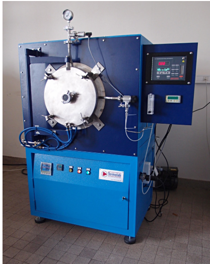
Figure 1: Chamber used for isothermal ageing at low oxygen percentage ( <0.1\% ), using an oxygen monitor and a low flow of nitrogen (0.1 standard litre per minute). The system is 1.4 m tall, 1.2 m wide.
