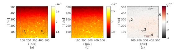
$F(\mathbf{r},t) = \log(f(\mathbf{r},t))$  and  $f(\mathbf{r},t)$  is the flat-field at time t. If the beam were steady,  $F(\mathbf{r},t)$  should be equal to  $F_i(\mathbf{r}) = \log(f_i(\mathbf{r}))$ , for all i. However, in the real life,  $F(\mathbf{r},t)$  varies in time as the X-ray beam is not steady. Since it is not possible to measure simultaneously I and F, one has to estimate  $F(\mathbf{r},t)$  from  $F_i(\mathbf{r})$ .
