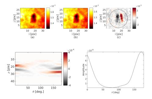
outside the circle shown in Fig. 4.2c d is set equal to 0), the Radon transform  $\rho = R[d]$  is computed and the mean quadratic intensity for every angle,  $l(\theta)^2$ , is computed as in Eq. (7). The results are displayed in figure 4.2. The minimum obtained in figure 4.2(b) gives the direction of the displacement:  $\theta \approx 80^{\circ}$  from the horizontal x-axis.
