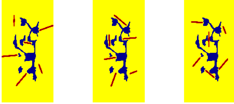
Figure 14: Optimally designed inclusion distribution topology for three 2D plates with multiple pre-existing cracks (cases 1-3 from left to right).
