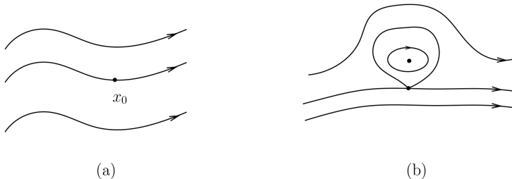
FIGURE 2.1. A schematic diagram of interior separation, (a) a parallel flow near x_0 , and (b) a vortex flow.
