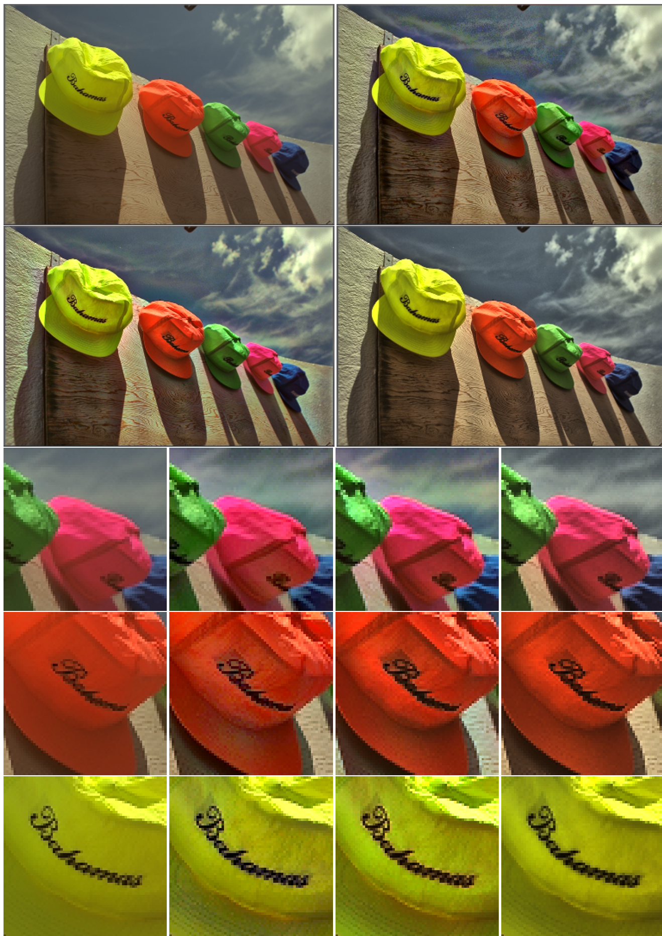
Fig. 8 Contrast enhancement of top-left image. Result given by the Euclidean model (29) in the RGB color space (top-right) and in the L^*a^*b^* color space (second row, left column). Result given by the model (31) induced by the connection 1-form (58) with the metric (74) encoding the Helmholtz-Kohlrausch effect (73) - Last three rows of the images on the top two rows: From left to right: Original image, Euclidean model (29) in the RGB and L^*a^*b^* color spaces, the model (31) induced by the connection 1-form (58) with the metric (74) encoding the Helmholtz-Kohlrausch effect (73).
