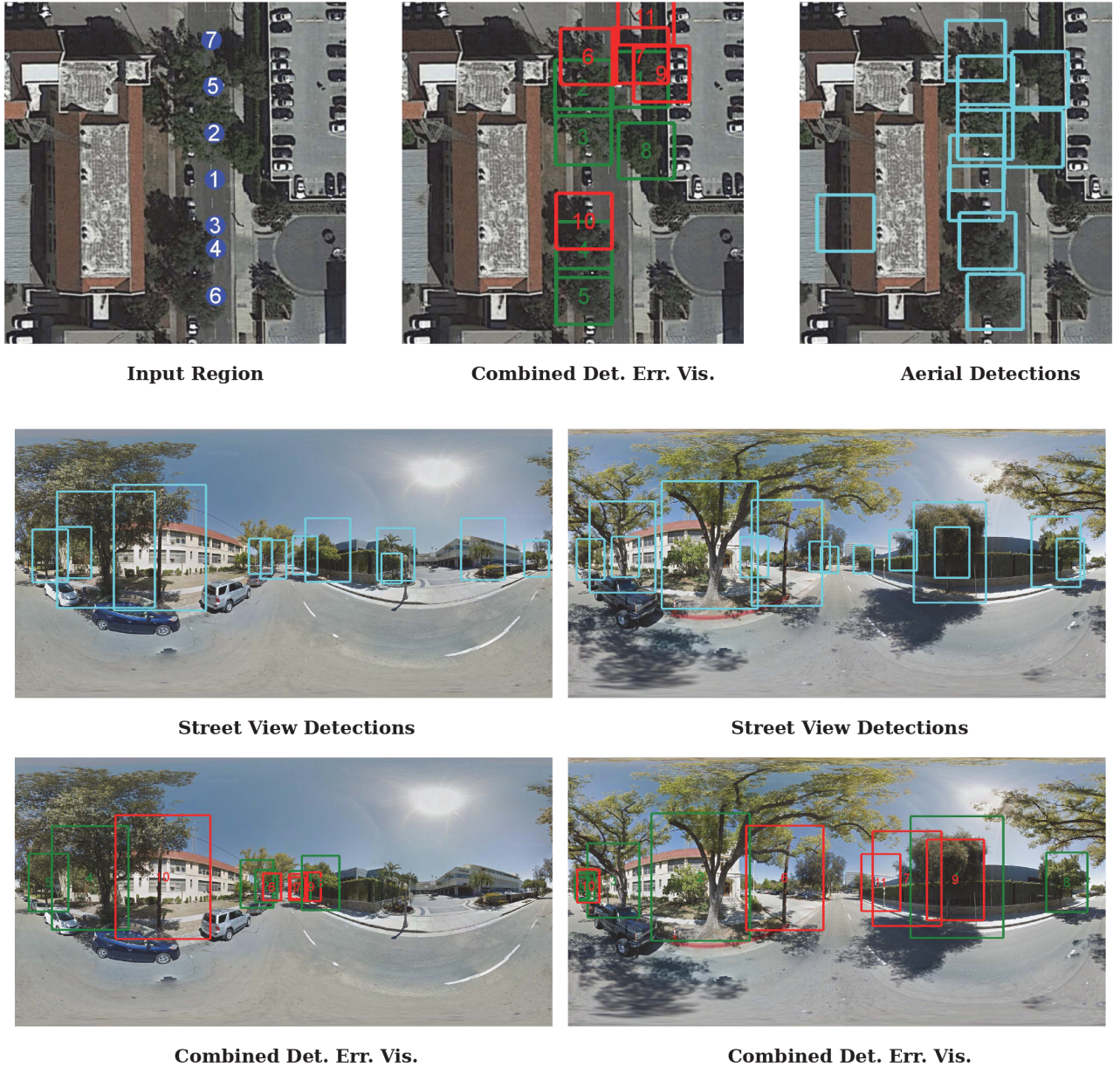
Fig. 8. Example for tree detection results (based on supplementary material of [6]): (top left) input aerial image with camera positions of the street-level panoramas (3 (left) and 5 (right) are shown below), (top center) aerial image overlaid with true positives (green) and false positives (red), (top right) tree detections based only on the aerial image, (middle left) tree detections based only on panorama 3, (middle right) tree detections based only on panorama 5, (bottom left) true positives (green) and false positives (red) overlaid to panorama 3 and (bottom right) panorama 5. Note that the panoramas in the bottom row and the aerial image top center show combined detection error visualizations.
