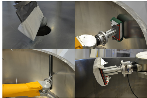
Fig. 7. Pictures of the prototype tools for scrubbing, scratching, evacuation and finishing.
