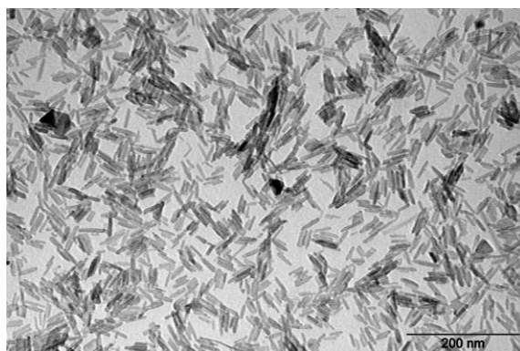
Figure 1: Transmission electron microscopy image of nanorods stabilized with Optima100
