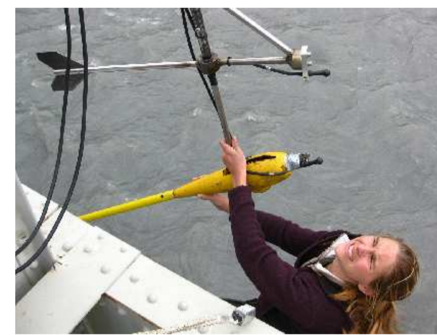
Fig. 6. Hydrophone deployment with sounding weight from a bridge on the Arc en Maurienne River.
