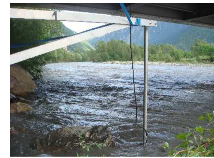
Fig. 8. Hydrophone deployment on a rigid structure from the bank of the Arc en Maurienne River.
