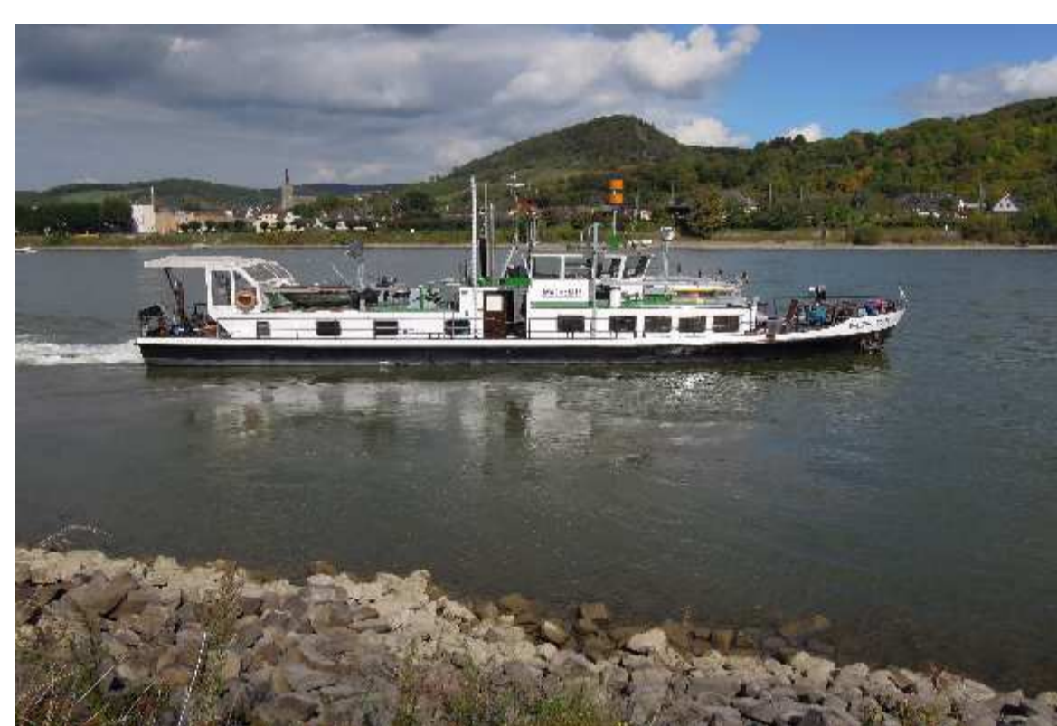
Fig. 2. Routine "MessSchiff" boat used for monitoring sediment. In the 300 m wide Koblenz cross-section of the Rhine, Germany.
