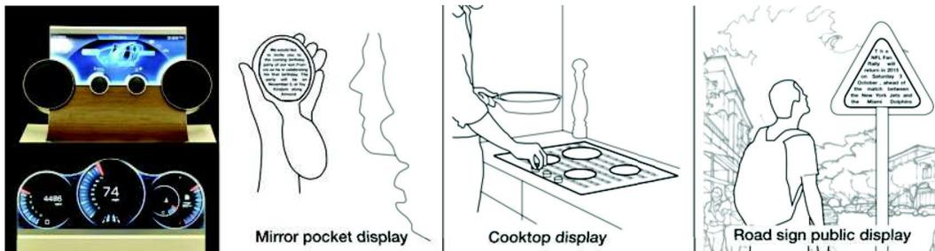
Figure 1. Left: Examples of freeform displays developed by Sharp. Right: Freeform display usage scenarios: circular mirrors for private notifications, shapes with holes such as a cooktop displays for recipes or the back of triangular road signs as public displays
