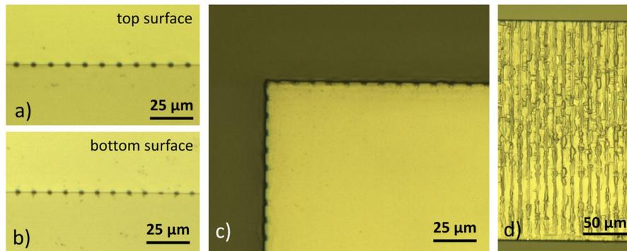
Fig. 5. Laser-induced cleaving of D263T glass by volume absorption of Bessel beams,  $E_p=70 \mu\text{J}$ , 4 pulses per burst,  $\theta_B=13.3^\circ$ , 10 kHz,  $v=125 \text{ mm/s}$ . a-b) microscopy images of laser entrance and exit surfaces, respectively. Black dots which result from initial laser modifications are joined by a thin crack on both surfaces. c) Top-view on the sample after cleaving reveals no chipping. d) Sidewalls have an average roughness  $R_a$  of less than 500 nm.
