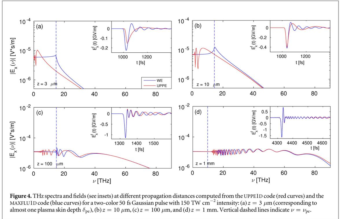
**Figure 4.** THz spectra and fields (see insets) at different propagation distances computed from the UPPE1D code (red curves) and the MAXFLU1D code (blue curves) for a two-color 50 fs Gaussian pulse with  $150 \text{ TW cm}^{-2}$  intensity: (a)  $z = 3 \mu\text{m}$  (corresponding to almost one plasma skin depth  $\delta_{pe}$ ), (b)  $z = 10 \mu\text{m}$ , (c)  $z = 100 \mu\text{m}$ , and (d)  $z = 1 \text{ mm}$ . Vertical dashed lines indicate  $\nu = \nu_{pe}$ .
