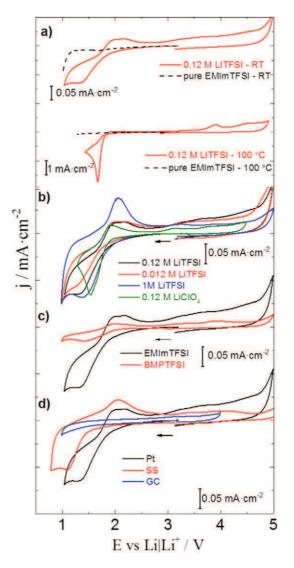
**Fig. 1.** a) The CV of pure EMImTFSI and 0.12 M LiTFSI solutions at RT (top curves) and 100 °C (bottom curves). The CVs of electrolyte containing Li<sup>+</sup> cations at RT b) different salt concentrations and salt anion WE - Pt<sub>p</sub> c) 0.12 M LiTFSI solution in different ILs, WE - Pt<sub>w</sub> d) 0.12 M LiTFSI solution in EMImTFSI on different electrodes. CE – Pt, RE – Ag|Ag<sub>2</sub>O, *sr* = 50 mV·s<sup>-1</sup>.
