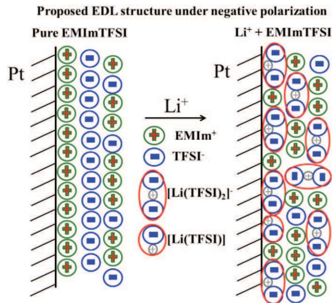
**Fig. 3.** The proposed schematic of EDL structure at negative polarization in pure ILs and after the addition of Li<sup>+</sup> cations.
