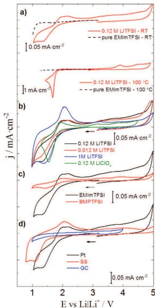
**Fig. 1.** a) The CV of pure EMImTFSI and 0.12 M LiTFSI solutions at RT (top curves) and 100 °C (bottom curves). The CVs of electrolyte containing Li<sup>+</sup> cations at RT b) different salt concentrations and salt anion WE - Pt<sub>p</sub> c) 0.12 M LiTFSI solution in different ILs, WE - Pt<sub>w</sub> d) 0.12 M LiTFSI solution in EMImTFSI on different electrodes. CE - Pt, RE - Ag|Ag<sub>2</sub>O, sr = 50 mV·s<sup>-1</sup>.
