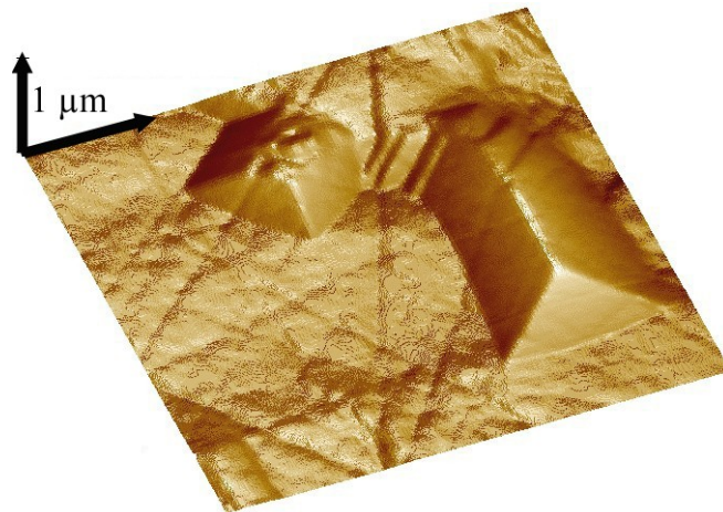
Fig. 3: Self accommodating martensitic variant pairs formed in the surroundings of a propagated crack of a double torsion test Ce-TZP sample.
