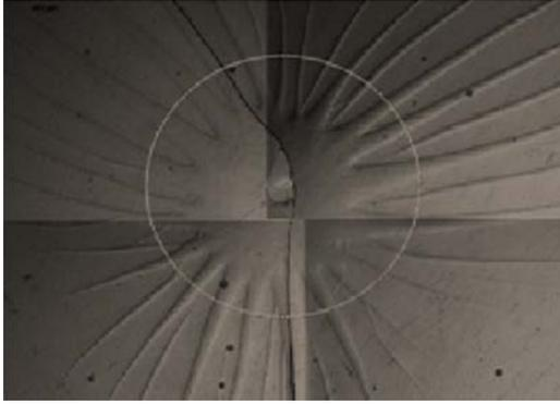
**Fig. 12 – Illustration of the transformation zone at failure. The circle corresponds to the effective surface for the POB configuration.**
