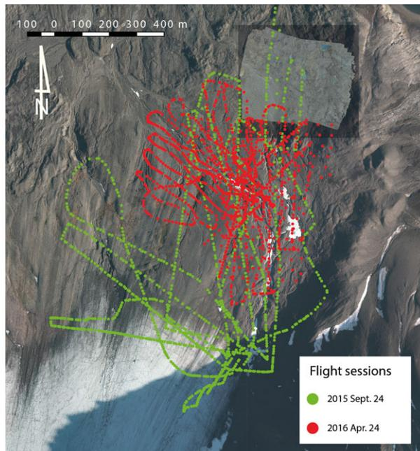
FIG. 3. Two manual flight paths for September 2015 and April 2016. The dots represent the GNSS position of each acquired photograph over features of interest.
