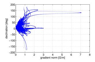
Figure 3. Estimated magnetic declination in inertial frame with respect to the gradient norm
