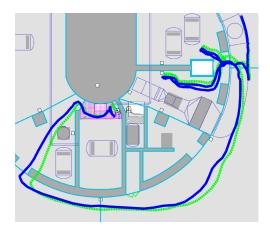
Figure 14. Trajectories estimated by the EKF (drashed green line) and the map-matching trajectory obtained by applying the particle filter on the EKF output (solid blue line).
