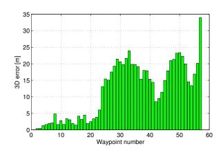
Figure 9. Distance from ground truth with the old algorithm. The third quartile of error is  $19.76 \mathrm{m}$
