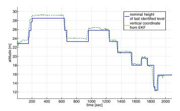
Figure 15. Altitude estimate of the magneto-inertial measurement unit (red curve) and the (nominal) altitude of the identified floor (blue curve) as a function of time for a course of 30 minutes through the labyrinth of the facility.
