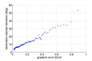
Figure 4. Declination standard deviation with respect to gradient norm
