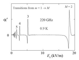
FIG. 2. The differential microwave absorption  $\alpha'$  at 220 GHz as the vertical holding field  $E_z$  was swept, showing resonant transitions from the ground state (sub-band), m = 1, to higher Rydberg states (sub-bands) m = M (with M up to 12 observed).
