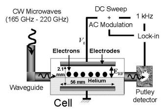
FIG. 1. Schematic diagram of the microwave cell. The cell was half-filled with liquid helium as a substrate for the surfacestate electrons. Vertically polarized microwaves were transmitted through the cell and detected by an InSb Putley detector. The vertical electric field  $E_z$  was swept through the microwave resonance. The field was a.c. modulated and the modulated microwave signal was detected using a lock-in amplifier.
