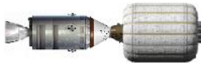
Figure 6: The ERV is composed of two modules: on the left is the wet propulsion system for the inbound trip with the Orion capsule and, on the right, the main habitat module for the return.
