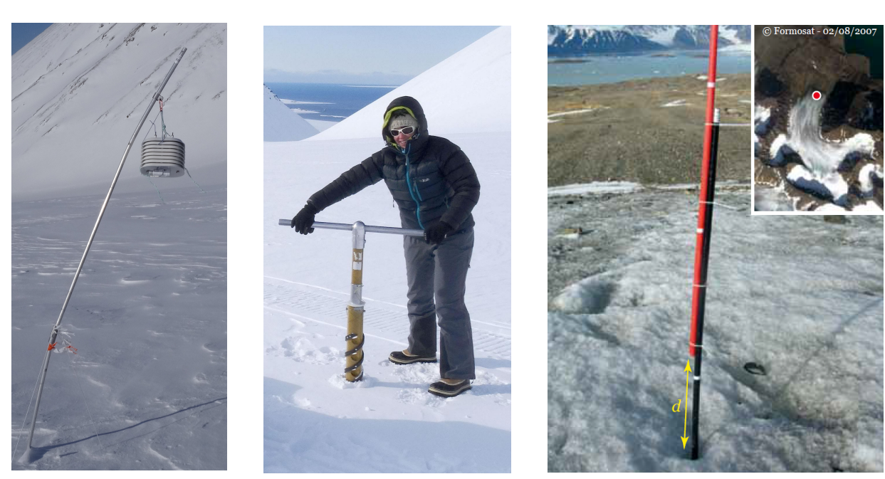
(b) 1. temperature sensor, 2. PICO drill, 3. ablation stake
