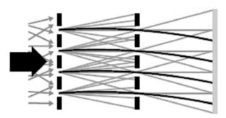
Fig. 3. The moiré deflectometer. The trajectories of un disturbed particles (grey lines) are modified by the presence of a force (black lines) and a shift of the fringe pattern occurs. In the case of gravity the shift  $\delta$  depends on both time of flight T and  $g\colon \delta=gT^2.$  g can be obtained by fitting the shift versus T on an event-by-event basis. The data will be recorded by means of a suitable detector placed in the third plane.
