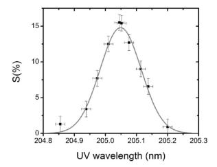
Fig. 5. Linewidth of the  $1^3S \to 3^3P$  Ps excitation as obtained by scanning the UV laser wavelength. Reproduced from Ref. [25].
