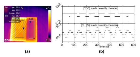
Fig. 3 a Snapshot of a radial surface taken with the IR camera as recorded during the experiments (right side covered with Advance black PVC tape and left side, uncovered) and  $\bf b$  conditions of temperature (°C) and RH (%) inside the humidity chamber during the experiments recorded with the data logger
