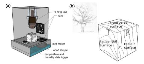
Fig. 2 a Experimental set-up showing (b) the three directions of wood (L for longitudinal, R for radial and T for tangential) and the corresponding surfaces (radial L-R, tangential L-T and transverse T-R)
