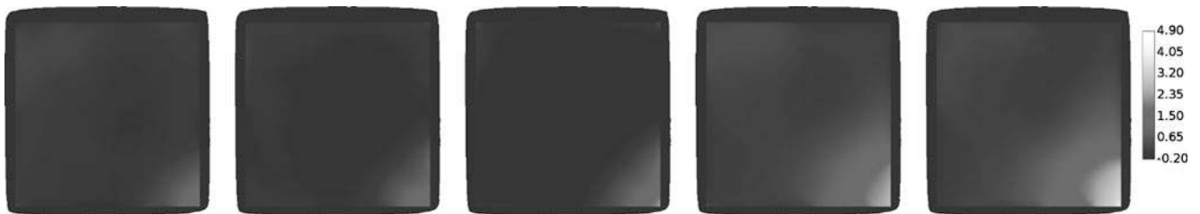
Fig. 28.6 Crack opening displacement evolution for the corner crack at 165 kc, 180 kc, 190 kc, 195 kc and 200 kc (scale in \mu\text{m} )
