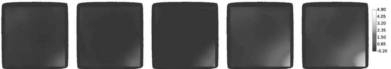
**Fig. 28.6** Crack opening displacement evolution for the corner crack at 165 kc, 180 kc, 190 kc, 195 kc and 200 kc (scale in  $\mu\text{m}$ )
