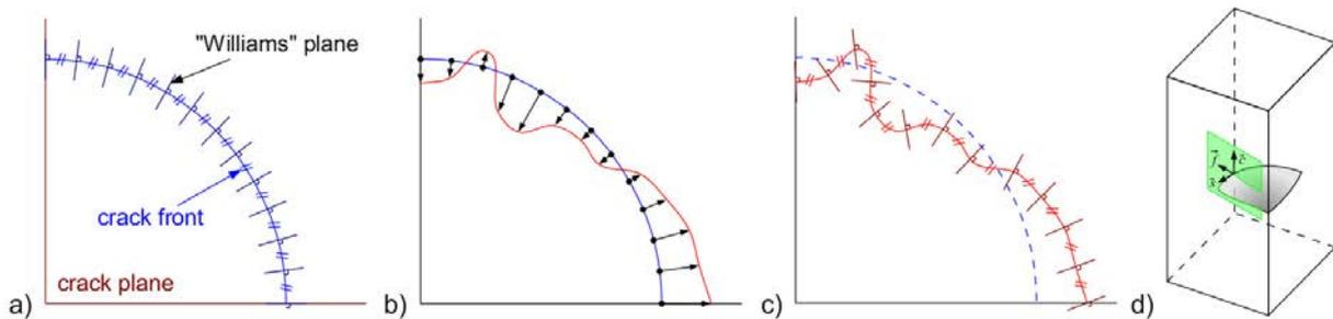
Figure 3: Schematic illustration of the iterative crack front extraction process : an initial crack front position is assumed (a) to build a series of planes which will be used for fitting the Williams series. Once the new position of the front is found (b) (see the text for details) a new series of planes is build (c) ; for non planar cracks, the process can be carried out in 3D (d).
