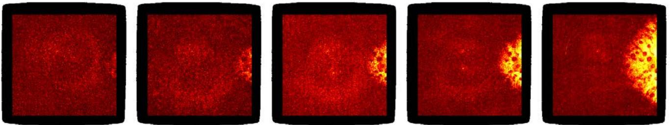
Figure 1: Surface crack evolution at 160 kc, 175 kc, 190 kc, 205 kc and 240 kc obtained from DVC residuals (the cross section of the sample is  $1.5 \times 1.5 \text{ mm}^2$ ).
