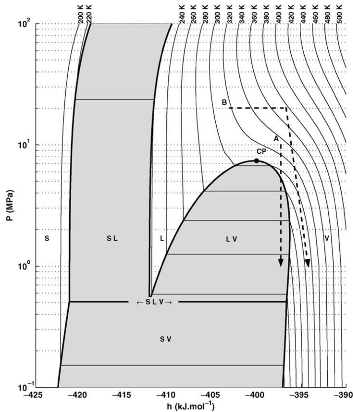
Fig. 2. Phase diagram of pure CO<sub>2</sub> (Peng-Robinson's model [6]).
