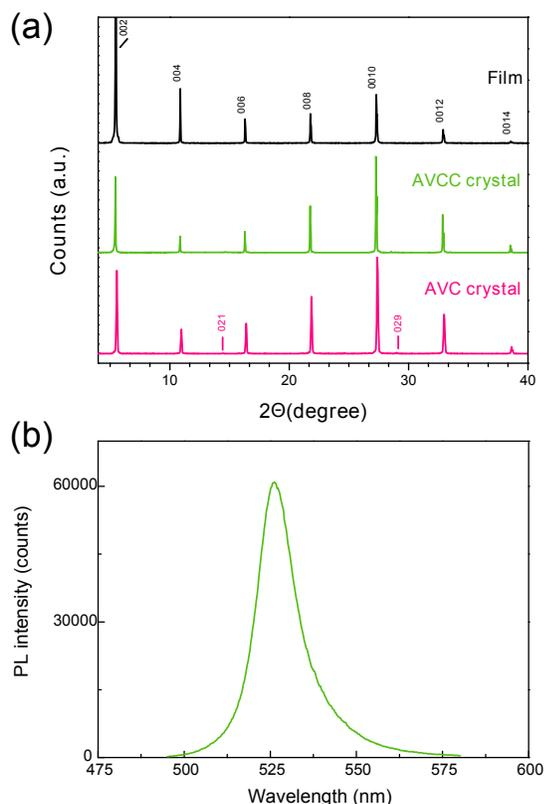
**Figure 2** (a) X-Ray diffraction patterns: standard PEPI thin film (black curve); AVCC crystal (green curve); AVC method (pink curve). (b) CW photoluminescence spectra of a AVCC crystal excited at 405 nm.
