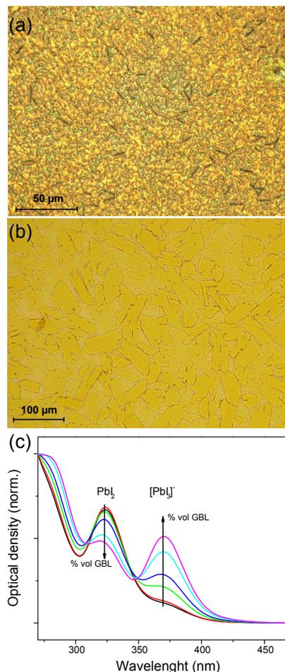
**Figure 3** Optical images of PEPI thin films (a) using DCM as solvent (b) using GBL as solvent. (c) Absorption spectra of  $10^{-3}$  mol.L<sup>-1</sup> PEPI solutions in DMF with an increasing amount of GBL from 10% vol (red curve) to 100% (purple curve).
