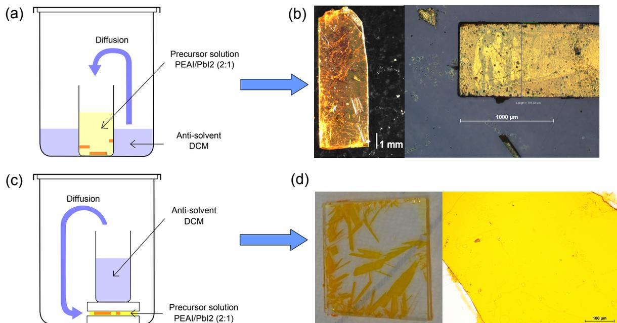
**Figure 1** (a) Schematic diagram of the AVC process (b) optical images of typical PEPI crystals obtained by AVC method. (c) Schematic diagram of the AVCC process. (d) optical images of PEPI crystals obtained by AVCC method. The size of the quartz plate is  $25\text{mm} \times 25\text{mm}$ .
