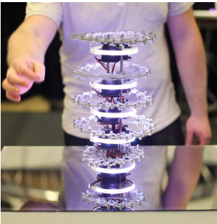
Figure 6: The actuated skeleton of AMPHORM (i.e. without its skin), a cylindrical kinetic sculpture [9].
