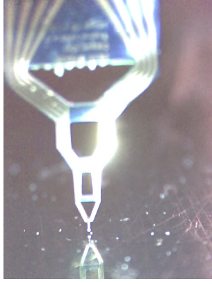
Figure 12: Hand-microscope picture of the cantilever probe as close to z = 0 as possible. The aluminum plate at z = 0 acts as a mirror, so that the sensor reflection can be seen. The actual distance to the bottom plate is less than 200 \mu\text{m} .
