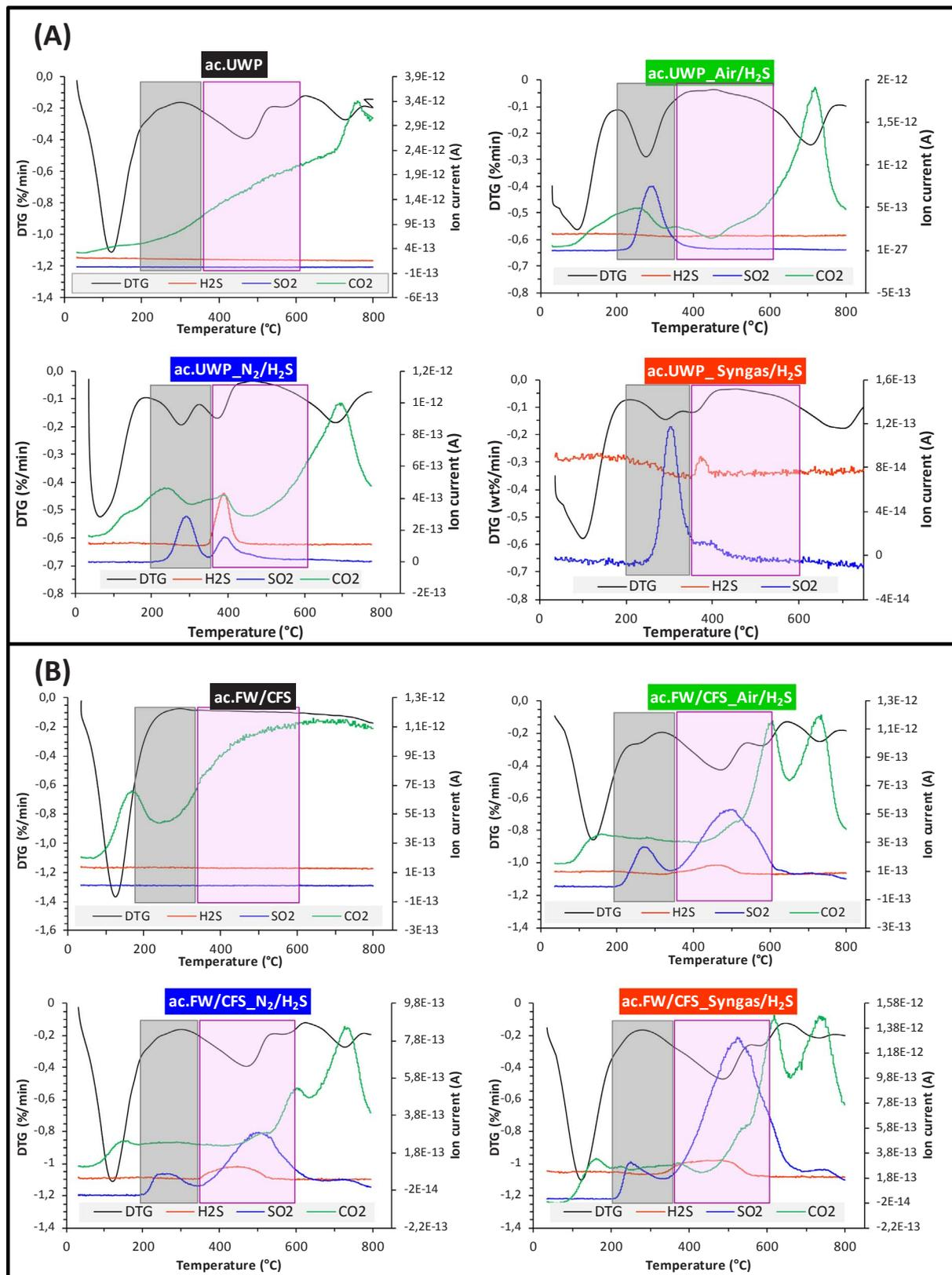
Fig. 3. TGA-MS analysis of ac.UWP (A) and ac.FW/CFS (B) before and after the H<sub>2</sub>S removal tests in different gas matrices.
