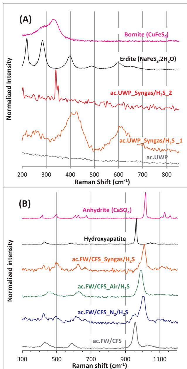
Fig. 4. Normalized Raman spectra of (A) ac.UWP, and (B) ac.FW/CFS before and after the H<sub>2</sub>S removal tests. Experimental spectra were compared with the RRUFF database spectra in order to identify the sulfur species formed.
