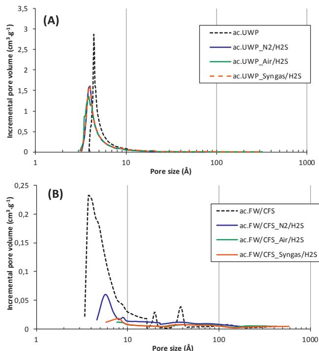
**Fig. 2.** Pore size distribution of (A) ac.UWP, and (B) ac.FW/CFS before and after the H<sub>2</sub>S removal tests in different gas matrices. The distributions were obtained using the Horvath-Kawazoe (HK) and the BJH (Barrett, Joyner et Halenda) methods after N<sub>2</sub> adsorption/desorption tests at 77 K.
