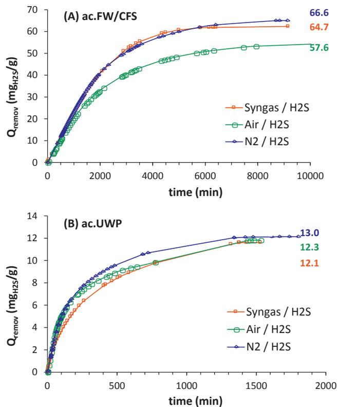
**Fig. 1.** Cumulative H<sub>2</sub>S removal capacity in different dry gas matrices of (A) ac.FW/CFS, and (B) ac.UWP.
