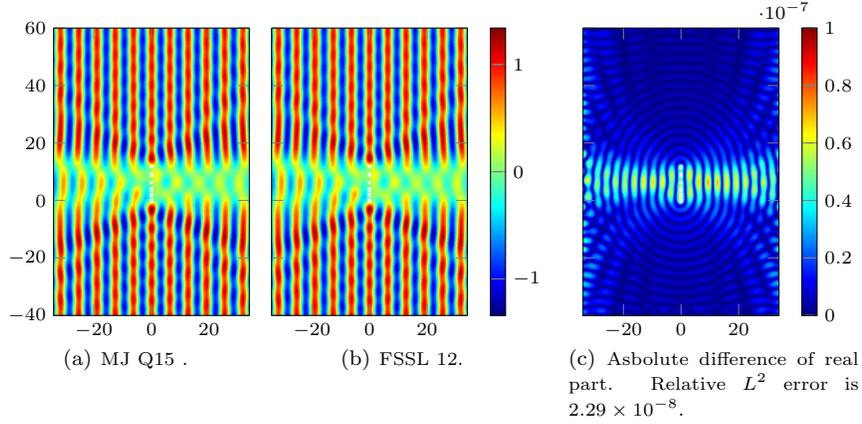
Figure 3: Real part of reference solution (total wave) in the soft-scattering of angle  $0^\circ$  PW with  $\lambda \sim 6.3$  by 6 obstacles with  $r = 0.4$  and  $2 \leq d \leq 2.9$ . (**Num. Exp. 1**)
