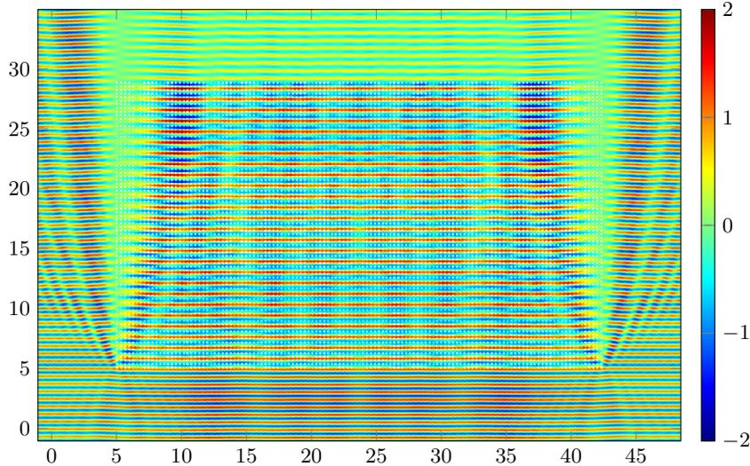
Figure 10: (Real part of) soft-scattered total wave of a PW of  $90^\circ$  with  $\lambda \sim 0.63$  by 10000 obstacles with  $r = 0.03$  and  $d = 0.3$ . FSSL approx order = 2. Matrix size =  $50000 \times 50000$ . Resolution by Scalapack on 48 processors. Visualization is  $800 \times 800$  grid on domain  $79\lambda \times 57\lambda$ . Total time  $\sim 25$  mins. (**Num. Exp. 6**)
